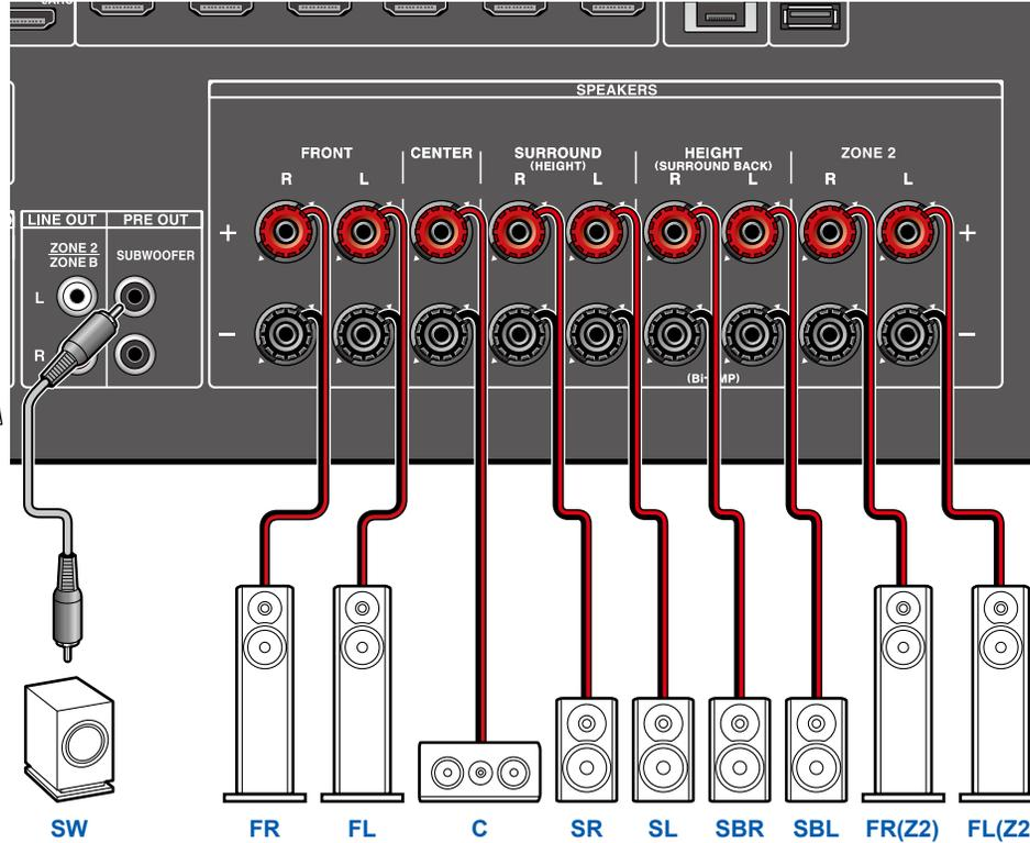
While ZONE 2 playback is being performed, surround back speakers installed in the main room cannot play audio.
