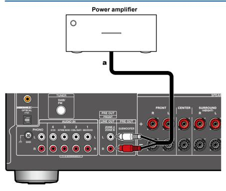
You can connect a power amplifier to the unit and use the unit as a pre-amplifier in order to produce a large volume that cannot be output with the unit only. Connect the front speakers to the power amplifier. For details, refer to the power amplifier's instruction manual.
