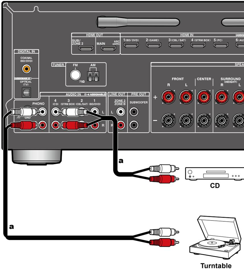
This is a connection example of an audio component. Connect a CD player using an analog audio cable. You can also connect a turntable that has an MM-type cartridge to the PHONO jack.
