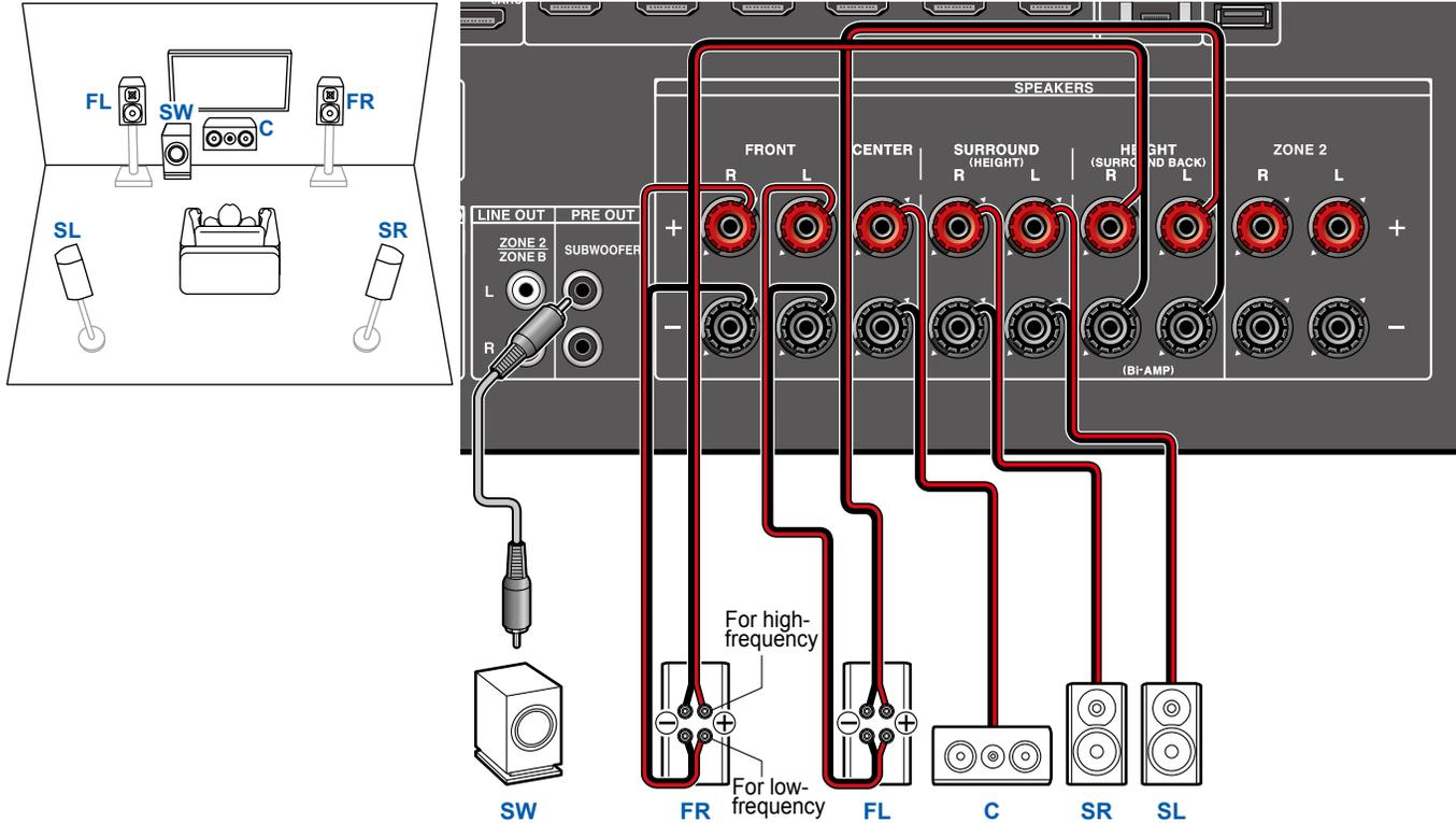
Be sure to remove the jumper bar connecting between the woofer jacks and tweeter jacks of the Bi-Amping supported speakers. Refer to the instruction manual of your speakers as well.
