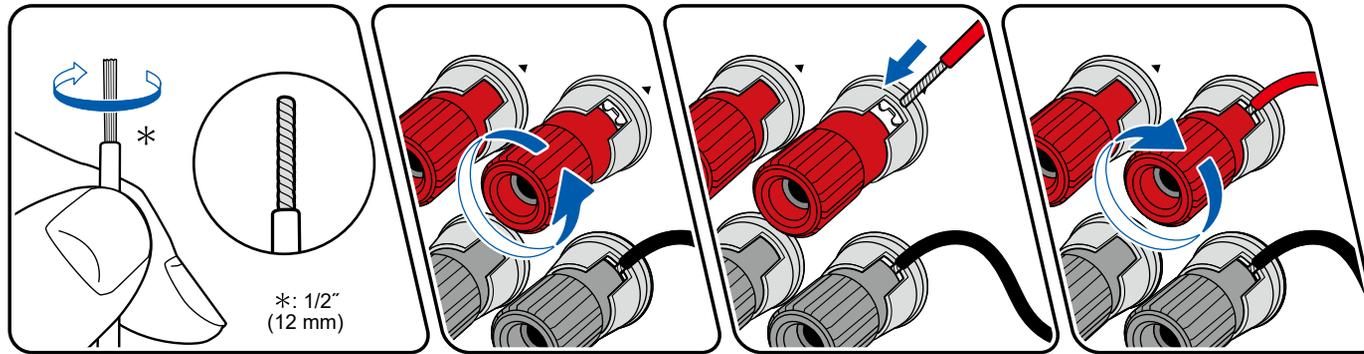
Make correct connection between the unit's jacks and speaker's jacks (+ side to + side, and - side to - side) for each channel. If the connection is wrong, a bass sound will not be reproduced properly due to reverse phase. Twist the wires exposed from the tip of the speaker cable so that the wires do not stick out of the speaker terminal when connecting. If the exposed wires touch the rear panel, or the + side and - side wires touch each other, a malfunction may occur.
