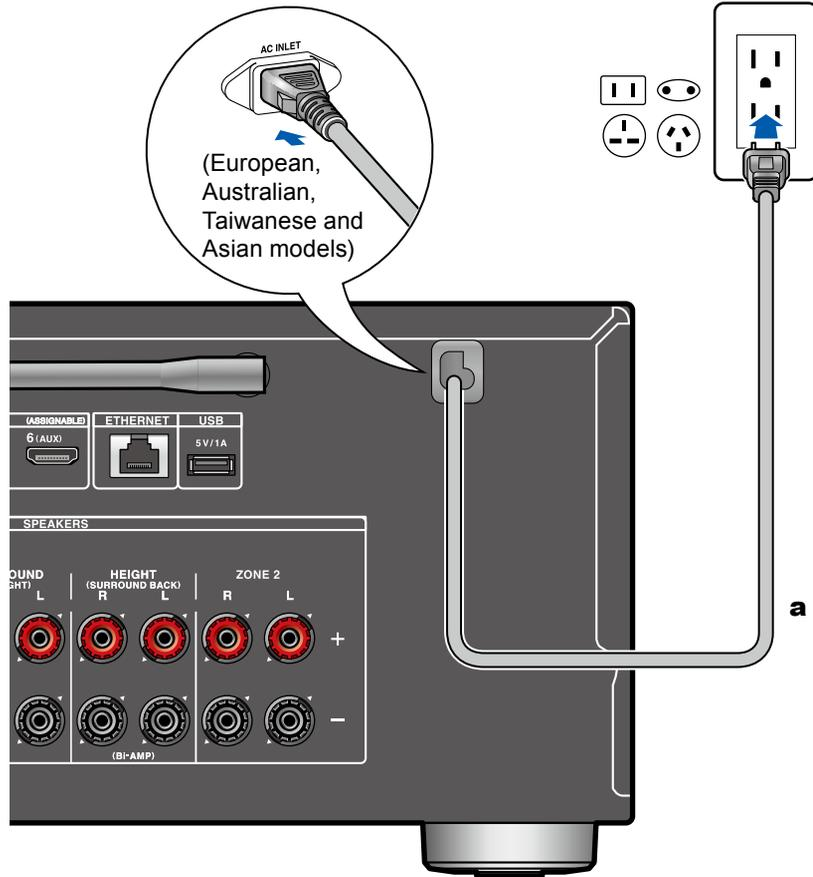
Connect the power cord after all the connections are completed.
