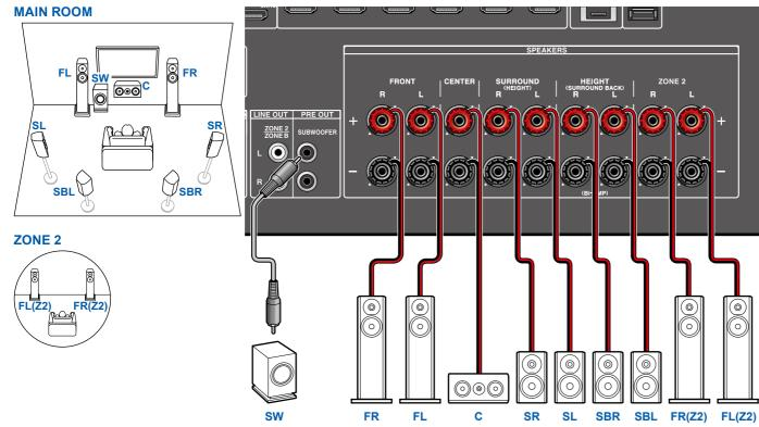
While ZONE 2 playback is being performed, surround back speakers installed in the main room cannot play audio.
