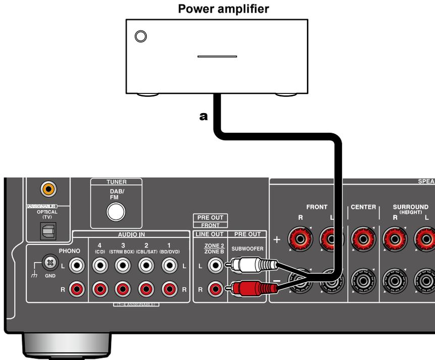
You can connect a power amplifier to the unit and use the unit as a pre-amplifier in order to produce a large volume that cannot be output with the unit only. Connect the front speakers to the power amplifier. For details, refer to the power amplifier's instruction manual.
