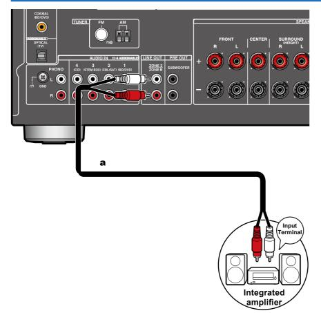
You can enjoy 2 ch audio in the separate room (ZONE 2) while performing playback in the main room (where this unit is located). Use an analog audio cable to connect the ZONE 2 LINE OUT terminal on this unit to the input jack on an integrated amplifier in the separate room.
