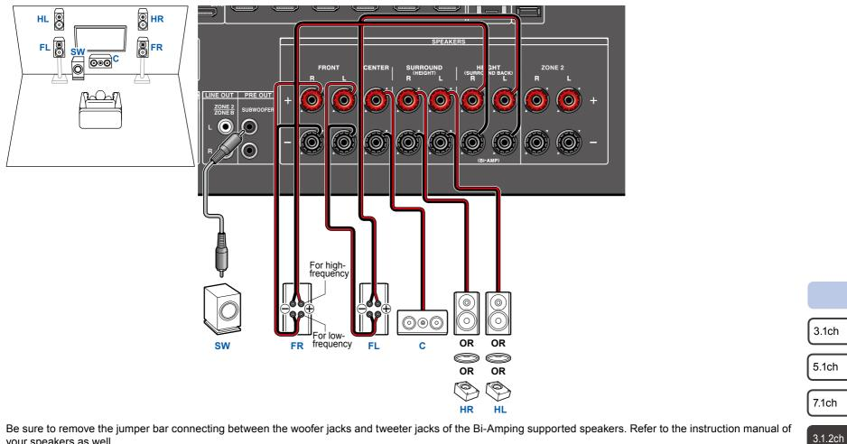
Be sure to remove the jumper bar connecting between the woofer jacks and tweeter jacks of the Bi-Amping supported speakers. Refer to the instruction manual of your speakers as well.
