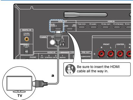
While a disc is played on a Blu-ray Disc player in the main room (where this unit is located), you can play the video and audio of the same Blu-ray Disc player or another AV component on the TV equipped with an HDMI IN jack in a separate room (ZONE 2). Note that only the devices connected to the HDMI IN1 to IN3 jacks can be played on the TV in the separate room.
