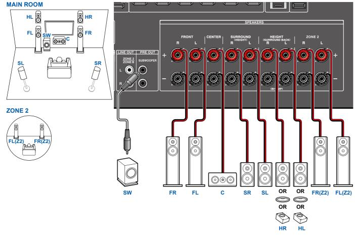
While ZONE 2 playback is being performed, height speakers installed in the main room cannot play audio.
