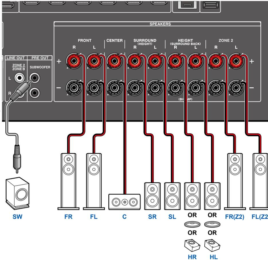
While ZONE 2 playback is being performed, height speakers installed in the main room cannot play audio.
