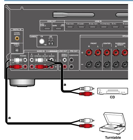
This is a connection example of an audio component. Connect a CD player using an analog audio cable. You can also connect a turntable that has an MM-type cartridge to the PHONO jack.
