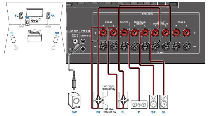
Be sure to remove the jumper bar connecting between the woofer jacks and tweeter jacks of the Bi-Amping supported speakers. Refer to the instruction manual of your speakers as well.
