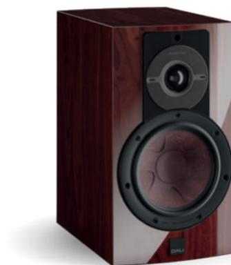
The **DALI RUBIKORE 2** stand-mount loudspeaker offers the ideal blend of compact size and generous sound. Its immensely rigid cabinet forms the perfect foundation to enable its ultra-light 29 mm soft dome tweeter and 6½ inch low-loss, Clarity Cone™ wood fibre driver to perform optimally. The result is a system characterised by intense clarity, expansive imagery and generous bass with both precision and timing.
