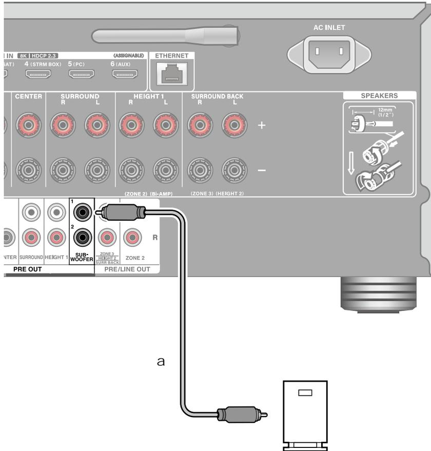
Connect a powered subwoofer with this unit using a subwoofer cable. Up to two powered subwoofers can be connected.
