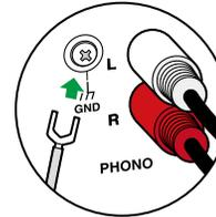
If the turntable has a ground wire, connect it to the GND terminal of this unit.
