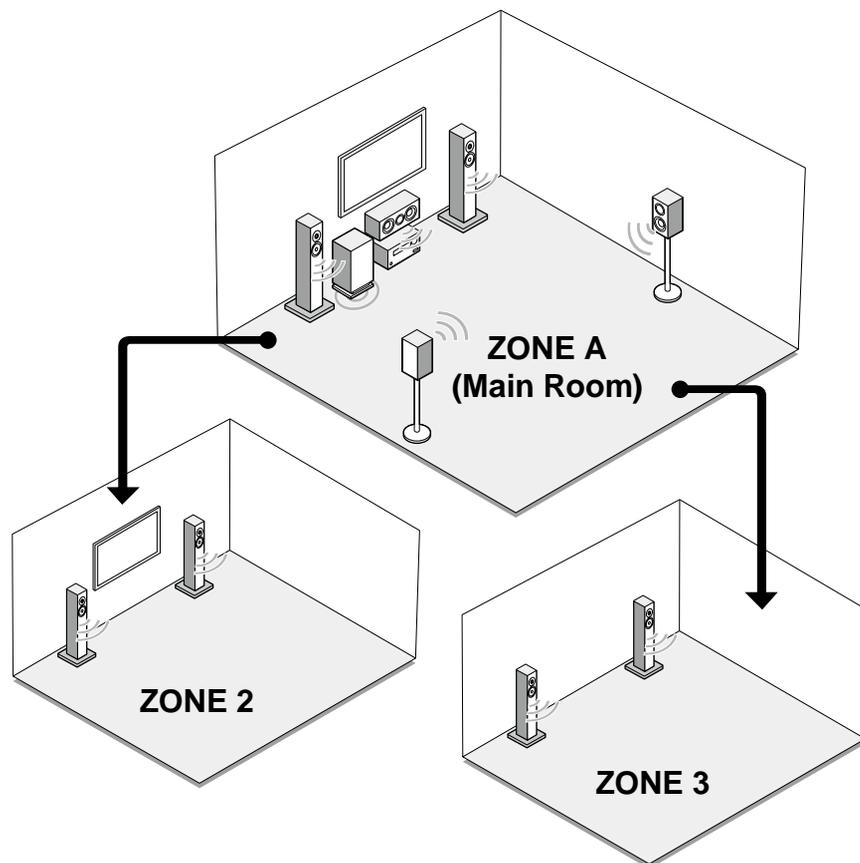
Using Onkyo Controller ( →[p143](#)) is convenient for operations of multi-zone playback. You can use it on mobile devices, such as a smartphone and tablet to which Onkyo Controller (available on iOS or Android™) has been downloaded.
