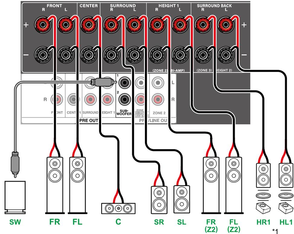
\*1 Connect the Height Speakers you have actually installed (HL/HR: Height Speakers, Top Speakers, Dolby Enabled Speakers).
