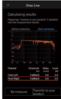
8. Disconnect the speaker setup microphone. The speaker adjustments based on the measurement results are saved in the unit. You can modify 3 patterns of the filter curves from the measurement results and register them in 3 slots (→[p146](#)). The filter curves that you register can be selected with "Room EQ" - "Dirac Live" (→[p75](#)) in "Quick Menu".
