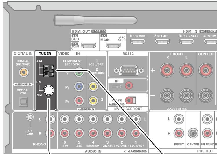
Connect the antenna to this unit, and set up the antenna at the best position for listening while receiving radio signals. Attach the indoor FM antenna to the wall using push pins or adhesive tape.
