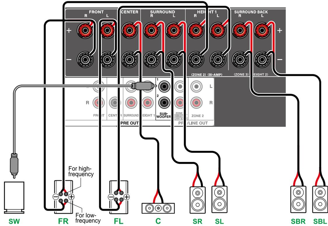
Be sure to remove the jumper bar connecting between the woofer jacks and tweeter jacks of the Bi-Amping supported speakers. Refer to the instruction manual of your speakers as well.
