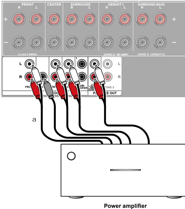
You can connect a power amplifier to the unit and use the unit as a pre-amplifier. This enables you to playback at high volumes that the unit by itself cannot produce. Connect the speakers to the power amplifier. For details, refer to the power amplifier's instruction manual.
