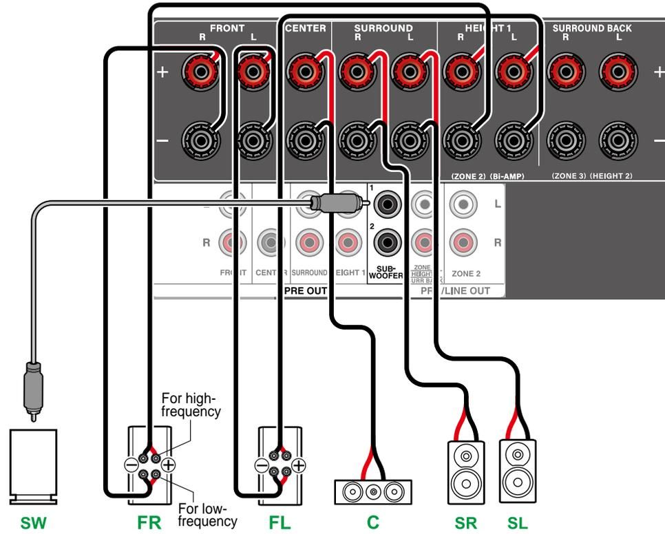
Be sure to remove the jumper bar connecting between the woofer jacks and tweeter jacks of the Bi-Amping supported speakers. Refer to the instruction manual of your speakers as well.
