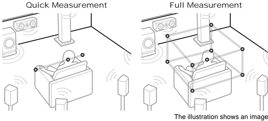
6. The guidance about outputting the test tone is displayed. Refer to the illustration to set up the speaker setup microphone in the listening position. Follow the on-screen instructions to measure.
