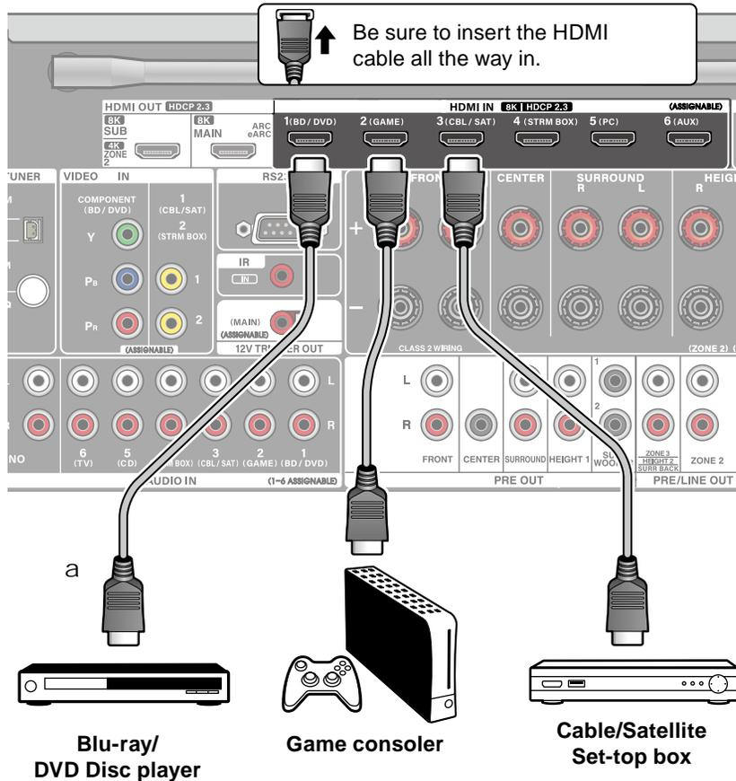
This is a connection example of an AV component equipped with an HDMI jack. When connecting with an AV component that conforms to the CEC (Consumer Electronics Control) standard, you can use the HDMI CEC function (\*) that enables linking with input selectors, etc. and the HDMI Standby Through function that can transmit video and audio signals of the AV component to the TV even if this unit is in standby mode.
