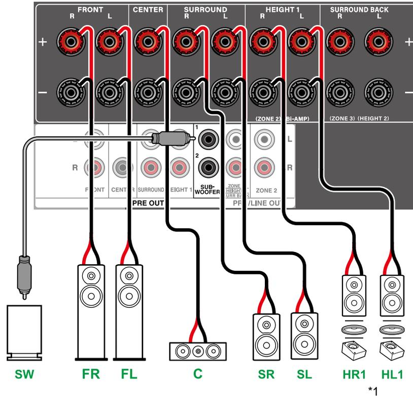
\*1 Connect the Height Speakers you have actually installed (HL/HR: Height Speakers, Top Speakers, Dolby Enabled Speakers).
