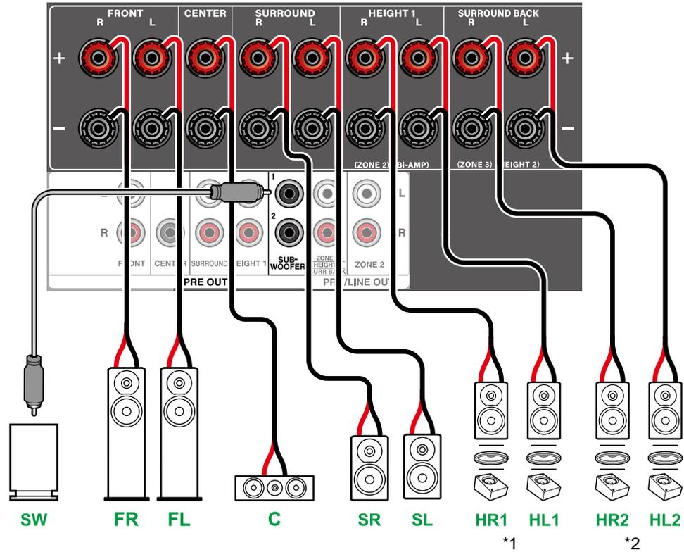
\*1 Connect the Height Speakers you have actually installed (HL1/HR1: Front Height Speakers, Top (front side) Speakers, Dolby Enabled Speakers (Front)).
