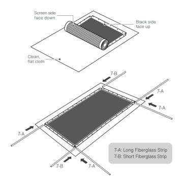
Put the assembled frames on the back side of the screen.
