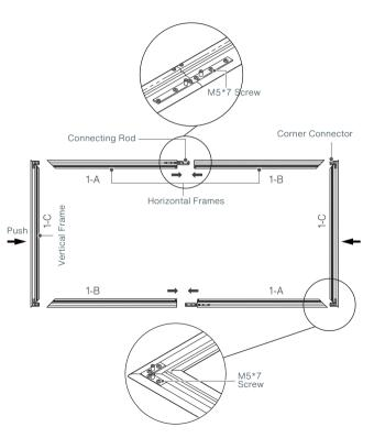
3. Install the support rod as shown below.
